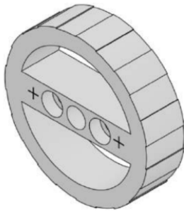
FIG. 2: Tungsten rotor CAD illustration (Figure 4.27 of [1]). Notice the shallow teeth on the outermost edge.
