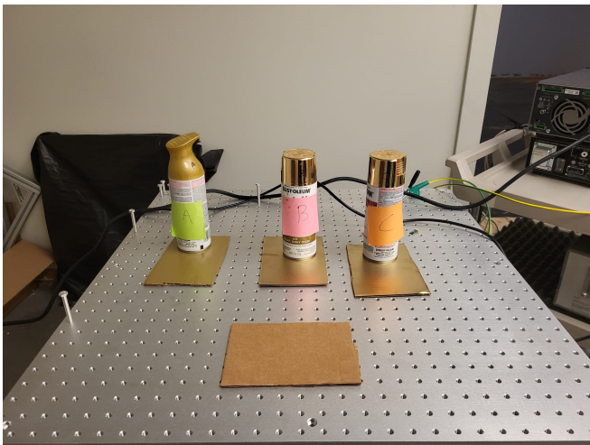
FIG. 4: The three paints chosen for this experiment atop their respective painted pieces of cardboard. The control (unpainted) piece of cardboard is pictured, as well. Each paint can is labelled from A through C with a post-it note. The cardboard pieces are labelled on their backs, as well.
