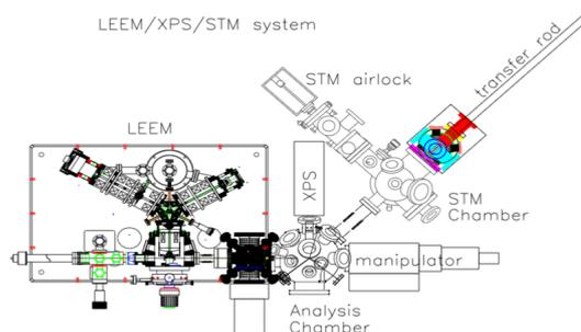
FIG. 2: UHV System. The system is composed of four interconnected chambers. Samples are placed in the system via the airlock and can be transferred to other chambers for cleaning and for LEEM, LEED, XPS, or STM analysis.
