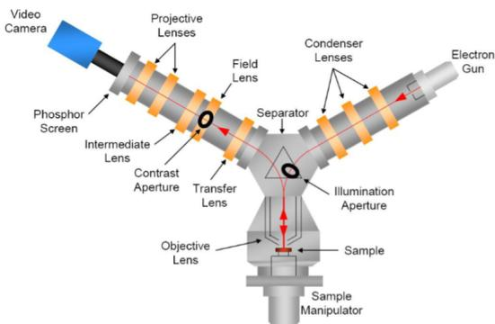
FIG. 1: LEEM and LEED. This is a diagram of the equipment used for LEEM and LEED analysis. It can be used for both real world imaging and taking diffraction images of samples placed into the UHV chambers.
