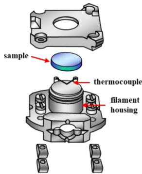
FIG. 3: Sample Holder Diagram. The sample holders are specially machined to be compatible with all measurement systems within the UHV system. The sample is secured above the thermocouple wires, which are attached to the feet of the holder. Underneath the sample is a housing for the filament which is used to heat the sample for cleaning.
