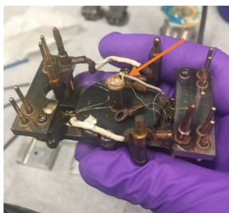
Fig 3. An STM scanner. The scanners perform vertical approach and can be removed from the instrument. The orange arrow indicates the location of the tube that holds tips. The tube is connected to a peg that allows a bias voltage to be applied.
