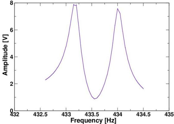
Figure 7: A frequency sweep of the wire when no vortex is present. As the excitation frequency approaches one of the resonant frequencies of the wire, the response amplitude increases forming a peak structure. The separation between these two peaks is a function of circulation.
