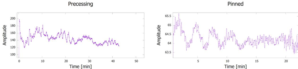
Figure 11: **Left:** The graph of response amplitude versus time shows a vortex precession in continuous mode. The period is consistent with precession in pulsed mode, and precession continues when switching between modes. This precession has higher frequency oscillations superimposed. **Right:** The graph of response amplitude versus time shows a pinned vortex in continuous mode. It features clear oscillations that may be Kelvin waves with higher frequencies superimposed.
