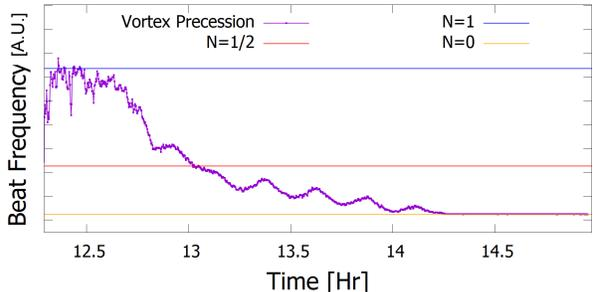
Figure 6: This graph of beat frequency versus time shows the precession of an off-center vortex over time. The maxima of these oscillations correlate to moments when the wire is closest to the cell wall and the most wire is covered by the vortex. These oscillations typically have a period of around 15 minutes.
