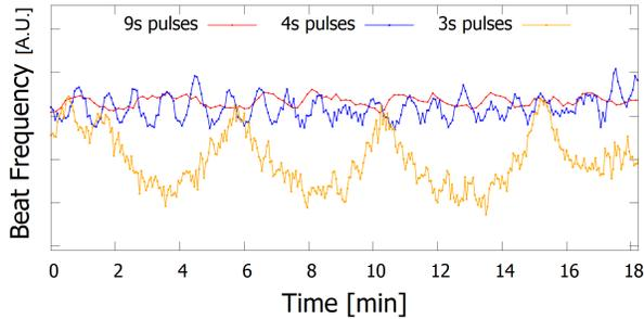
Figure 9: This graph of time versus beat frequency shows the behavior of a pinned vortex in pulsed mode. The red line represents data taken with nine second pulses while the blue line represents four second pulses. The blue line shows clearer Kelvin waves with higher frequency oscillations superimposed. The yellow line shows three second pulses, which result in a clear dip pattern superimposed over the Kelvin waves. The curves are shifted in time to overlap.
