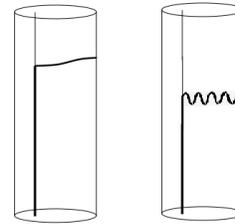
Figure 4: Left: A diagram of the vibrating wire cell when the vortex core detaches from the wire and extends instead to one of the cell walls. [2]. Right: A sketch of Kelvin wave vibrations on the free vortex core.
