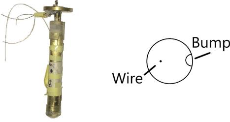
Figure 2: Left: An image of the vibrating wire cell before it is mounted on the fridge. The cell is about 3 inches long and 1.5 inches in diameter. The wire spans it vertically under tension. The bump is located about halfway down the side of the cell. Right: A schematic of a top-down view of the vibrating wire cell. The wire runs through the middle and the bump is attached to the cell wall.
