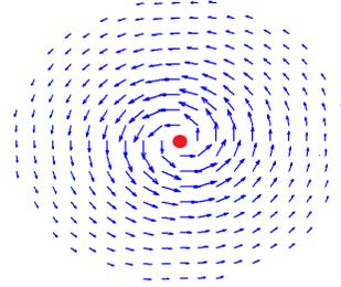
Figure 3: A diagram of a  $1/r$  velocity field like the one that surrounds the vibrating wire. In this schematic, the wire, represented by the red circle, passes perpendicularly through the field into the page.
