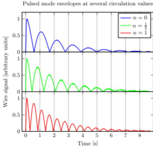
Figure 5: Pulsed mode envelope decays with varying circulation values. In the top data set, there is no circulation while in the bottom two, a vortex covers half and all of the wire respectively. As the circulation increases, the beat frequency also increases. The circulation values can be determined from these decays using a fitting function. [6]
