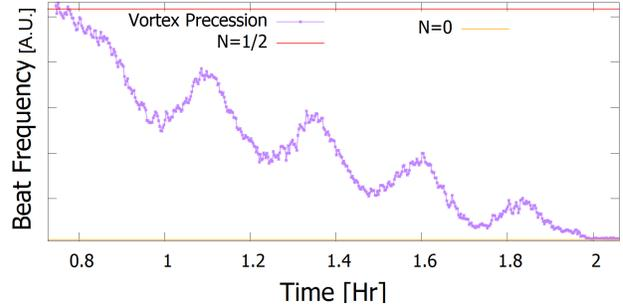
Figure 10: This graph of beat frequency versus time shows vortex precession, with a period of about 0.25 hours, as well as additional higher frequency oscillations that are thought to be Kelvin waves.
