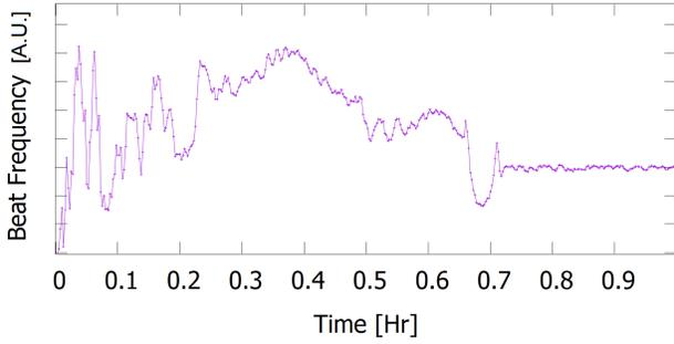
Figure 8: This graph of time versus beat frequency shows a clear signature as the vortex pins on the sty-cast bump at around 0.65 hours. The beginning part of the graph shows precession followed by a broad dip leading to a nearly horizontal line once the vortex pins. This signature was observed repeatedly when the vortex pinned.
