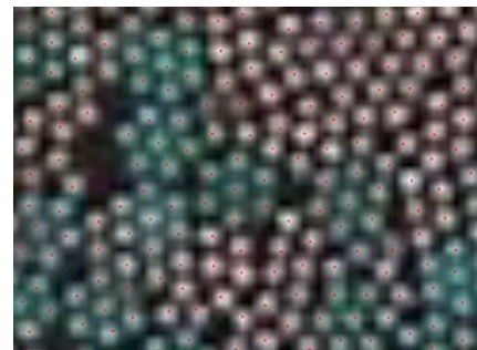
Fig. 3. In this image the program is identifying the brightest spot in the balls and is labeling them as ball centers (red dots).
