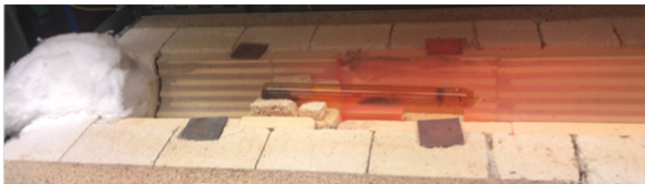
Figure 10. MM147 \text{Hf}_2\text{Te}_2\text{P} with selenium in the chemical vapor transport furnace. The temperature increases left to right.
