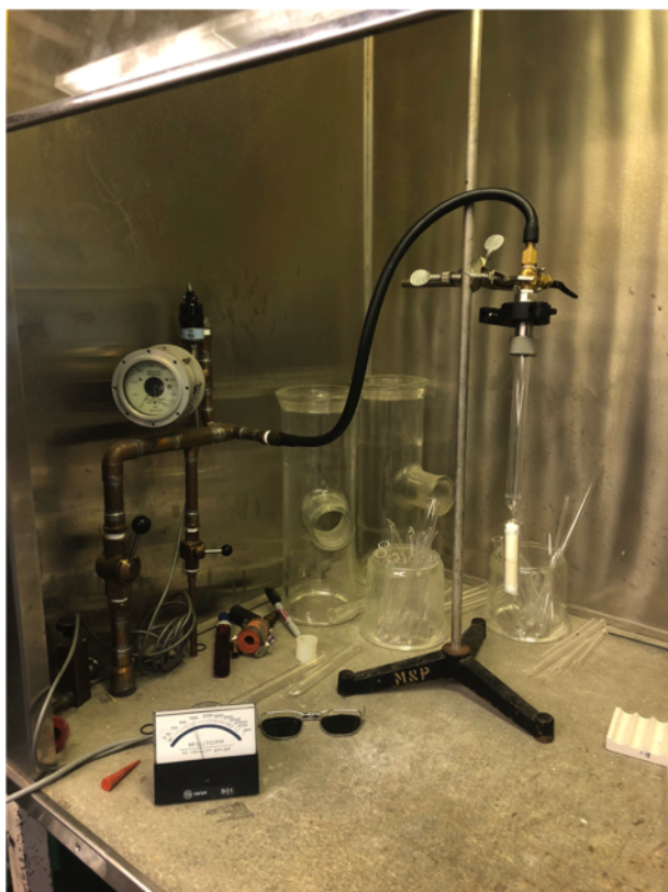
Figure 5. Sealing an ampoule. The necked ampoule is attached to a vacuum pump and argon gas tank. The ampoule is alternatively put under vacuum and backfilled with argon to purge impurities from the sample and ampoule.
