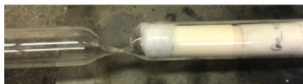
Figure 4. Necked ampoule. Quartz wool and crucible with unreacted elements to the right, empty ampoule in the left.
