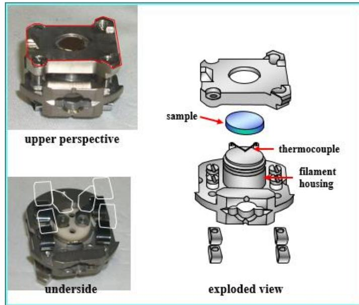
Figure 4. Images of a sample holder from the top (top left) and bottom (bottom left). Included is an expanded diagram of the sample holder (right)
