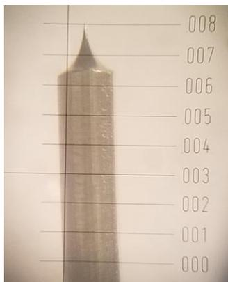
Figure 8. An image taken through a microscope of a chemically etched tungsten tip. The markers on the right indicate millimeters
