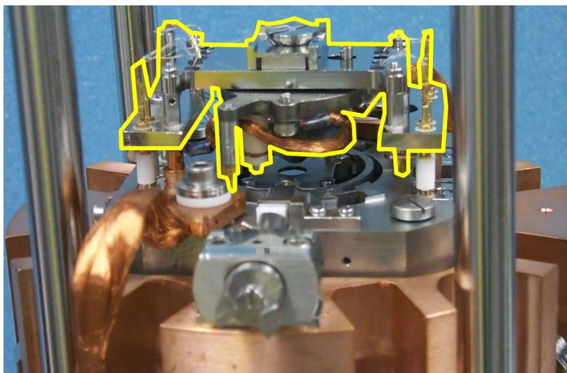
*Figure 2. The scanner (outlined in yellow) in its place on the copper block. The copper block is roughly 10 inches in diameter.*
