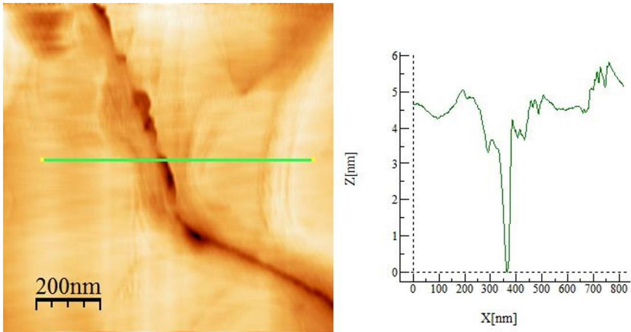
Figure 11. On the left is the image recorded by the STM after some noise was removed. This is a feature formed in a gold film deposited on a mica surface. The size scale is indicated in the bottom left corner. The green line indicates where the data on the right comes from. This graph shows the height ( $Z$ ) versus the horizontal position ( $X$ )
