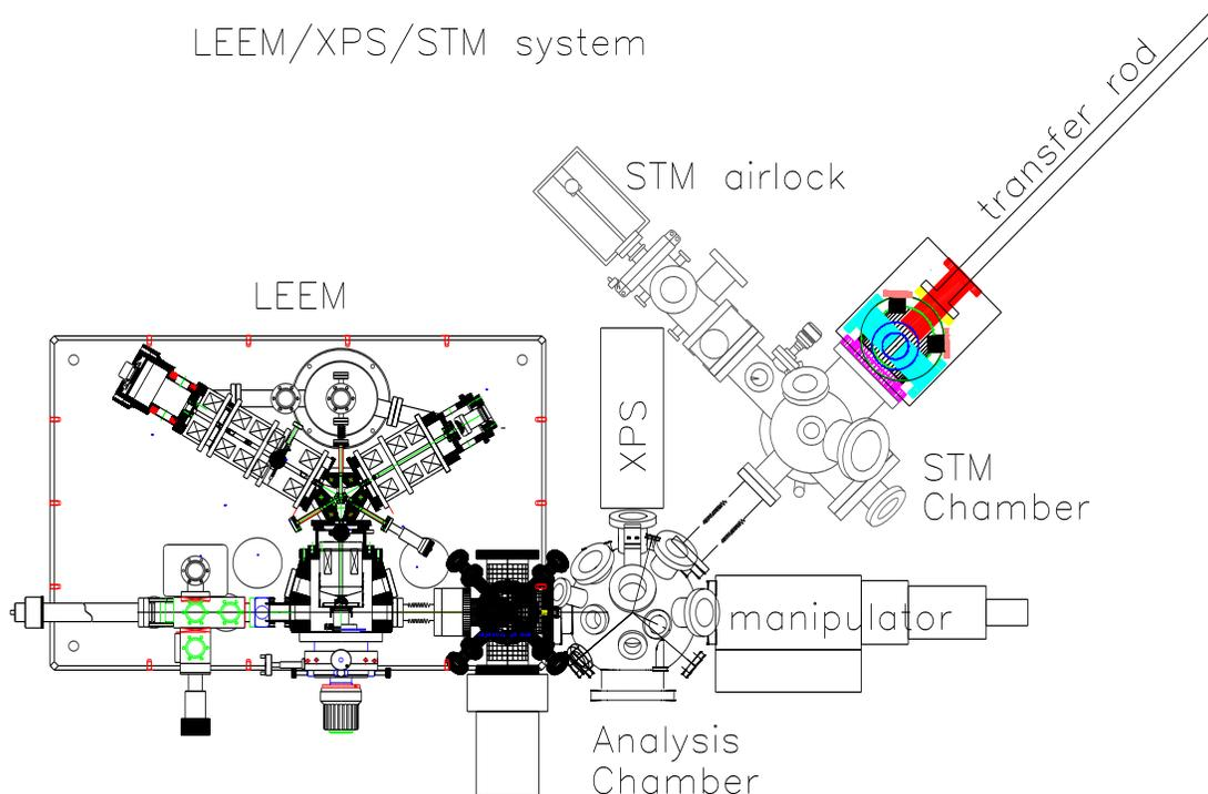
Figure 1. Diagram of the apparatus used as seen from above.
