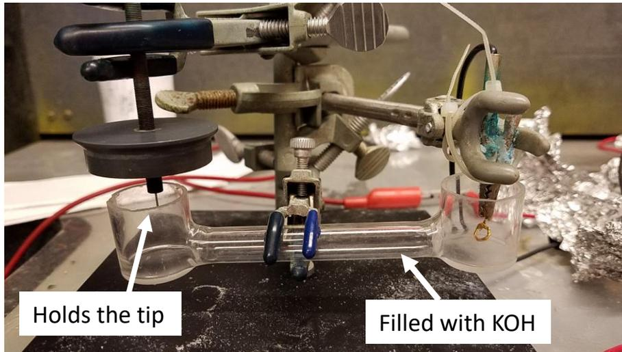
Figure 9. The equipment used to chemically etch the STM tips
