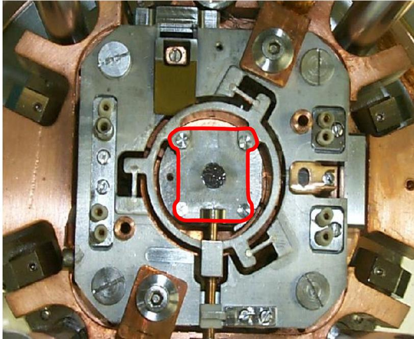
*Figure 3. The sample holder (outlined in red) secured in place in the copper block. The copper block is roughly 10 inches in diameter.*
