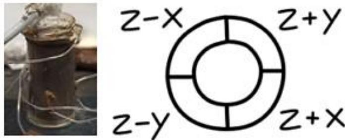
Figure 7. On the left, is a close-up of the piezoelectric tube. On the right, a diagram of the quadrants of the piezo, as seen from above. Each quadrant is electrically isolated from the others.
