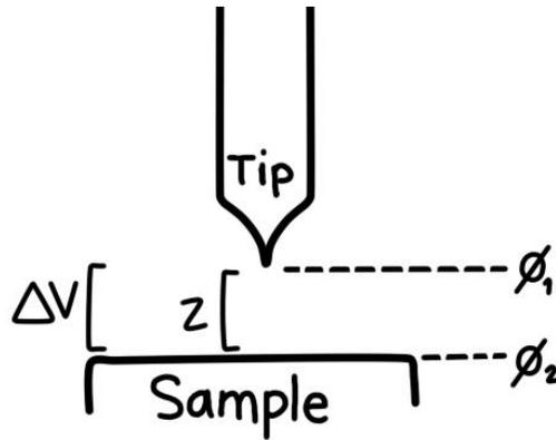
Figure 10. A diagram of the tip and the sample, showing the variables used in the equation to find the distance between the tip and the sample.
