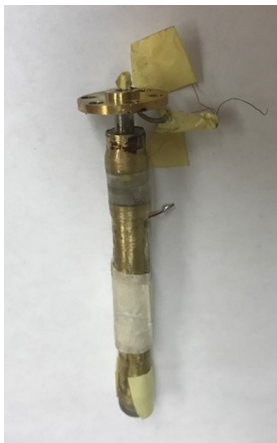
FIG. 2: A picture of the cell. The length of the brass cell is approximately 2-3in. A thin superconducting wire goes through the cell and comes out the stycast caps as a thick stranded wire. The top piece, known as the base, consists of a brass piece, copper-nickel tube, and stycast block. The tube and block allow the connection of the wire to the fridge. The base uses an indium O-ring and screws to secure the cell to the fridge.
