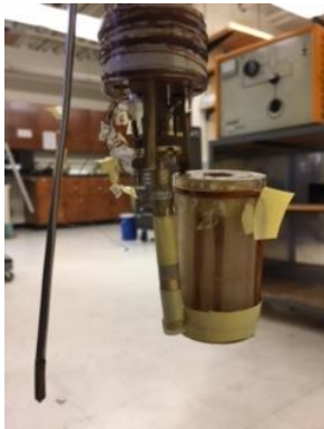
FIG. 2: Here the cell is attached to the fridge and the cylinder to the right contains the magnets.
