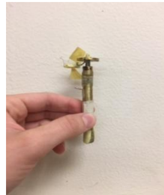
FIG. 1: Here is a fully assembled cell which will be attached to the fridge and filled with superfluid helium.
