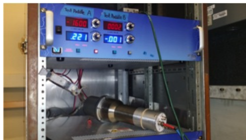
Figure 3: Experimental setup for the energy calibration of EJ-301.
