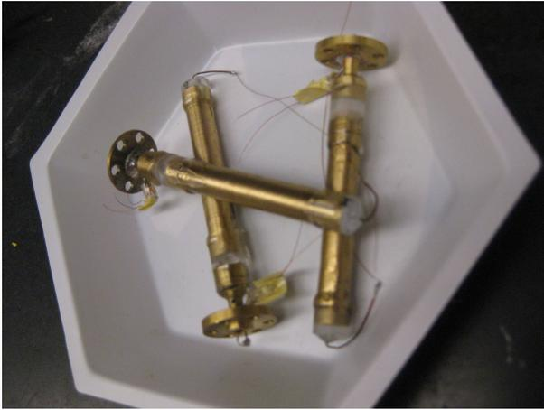
Figure 11: A photograph of three completed cells, including brass attachments that allow them to be screwed on to the cryostat. One of these is from a few years ago; I built the other two.
