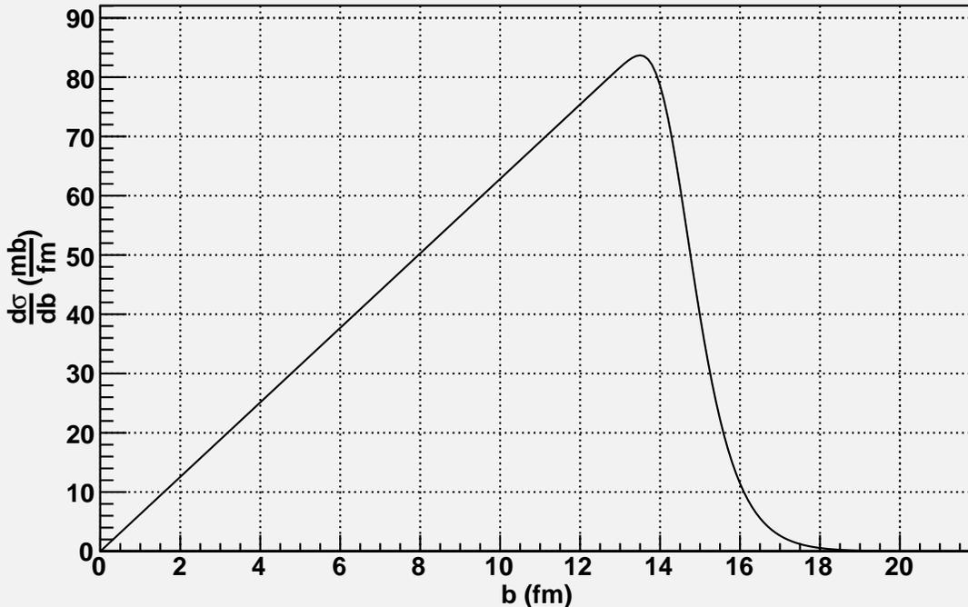
Figure 2: This is a plot of the geometric cross-section -vs- $b$  for Au. As the impact parameter increases, the probability of having an event increases.
