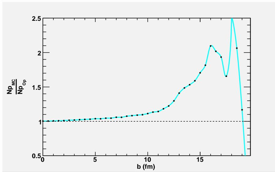
Figure 5: This is a plot of the ratio of the Monte Carlo over the Optical participant multiplicity. Observe how this ratio is greater than one at all impact parameters.
