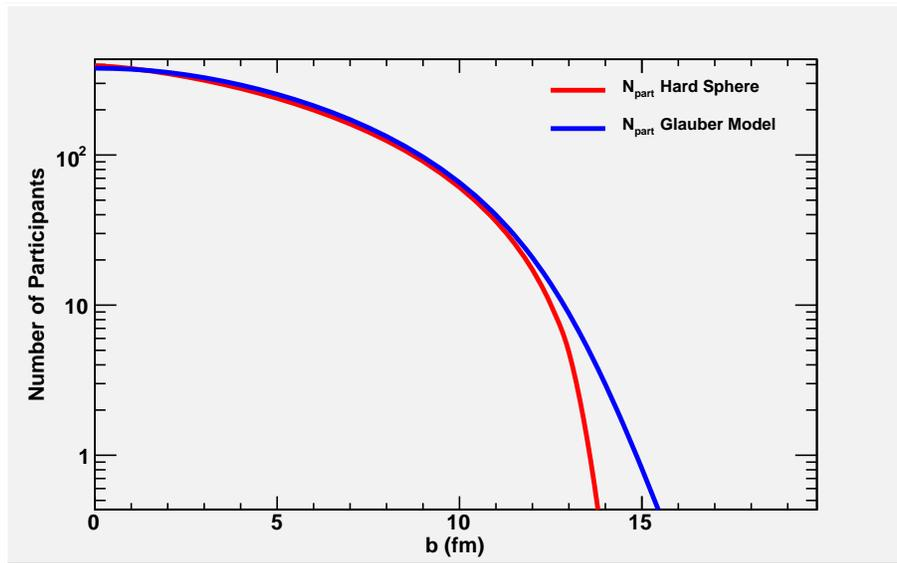
Figure 3: This is a plot of the participant multiplicity found using the Hard Sphere Approximation and the Optical Glauber Model.
