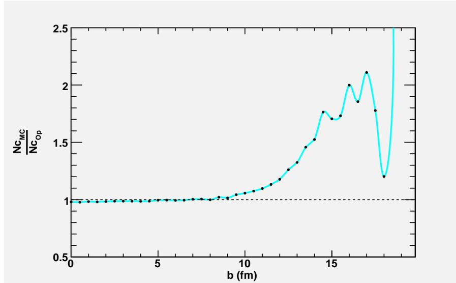
Figure 7: This is a plot of the ratio of the Monte Carlo over the Optical collision multiplicity. Observe how this ratio is greater than one at most impact parameters.
