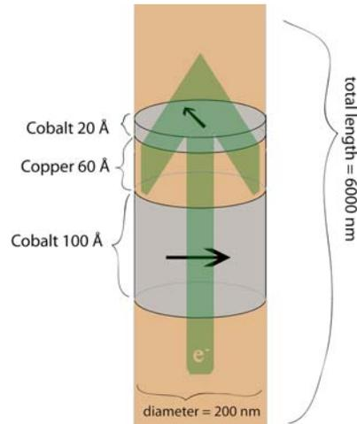
Fig.1: Current-induced switching in a Co/Cu wire. The upper cobalt layer will align with the lower if the current density is high enough.
