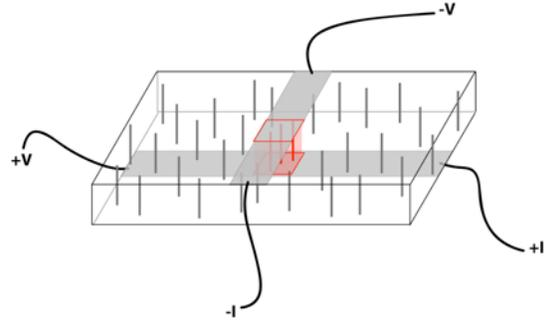
Fig. 3: Silver cross-leads on a sample. Only the center wires (red area) conduct through.
