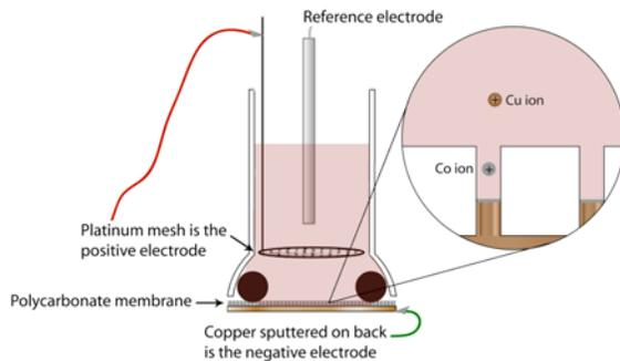
Fig. 2: Electrodeposition apparatus. Cobalt or copper ions fill the pores depending on the applied voltage [5].
