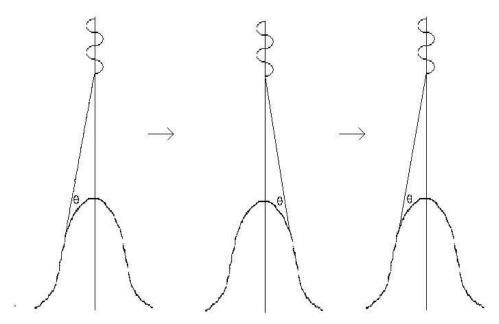
[Figure] – The sine wave oscillation is due to the wire's circular vibration and the magnets' alignments.
