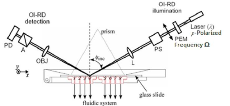
Figure 1: Schematic of an OI-RD microscope with a prism for total internal reflection. The microchip is mounted in a metal clasp, the reaction chamber, which holds the microarrays in position against the fluidics system. PEM, photoelastic modulator for modulating polarization; PS, phase shifter; L, focusing lens; OBJ, objective lens for facilitating detection; A, polarization analyzer; PD, photodiode detector.
